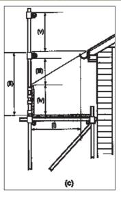
Sloping roof edge protection; Typical arrangement in conventional tube and fittings: (b) Working platform below the
