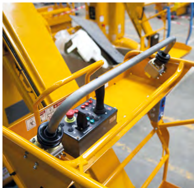
Haulotte Activ'Shield Bar (anti-entrapment system)
